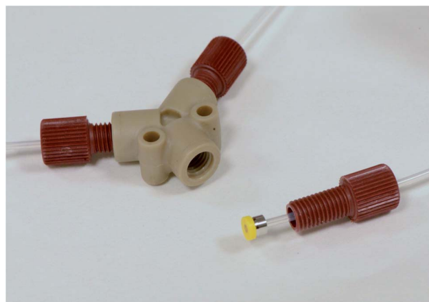
Fig. 1 Photograph of a microfluidic Y-mixer, with the outlet opened to reveal a yellow ferrule attached to the end of a length of PTFE tubing. The ferrule forms a liquid-tight seal with the Y-mixer when pressed into place by the red nut.
