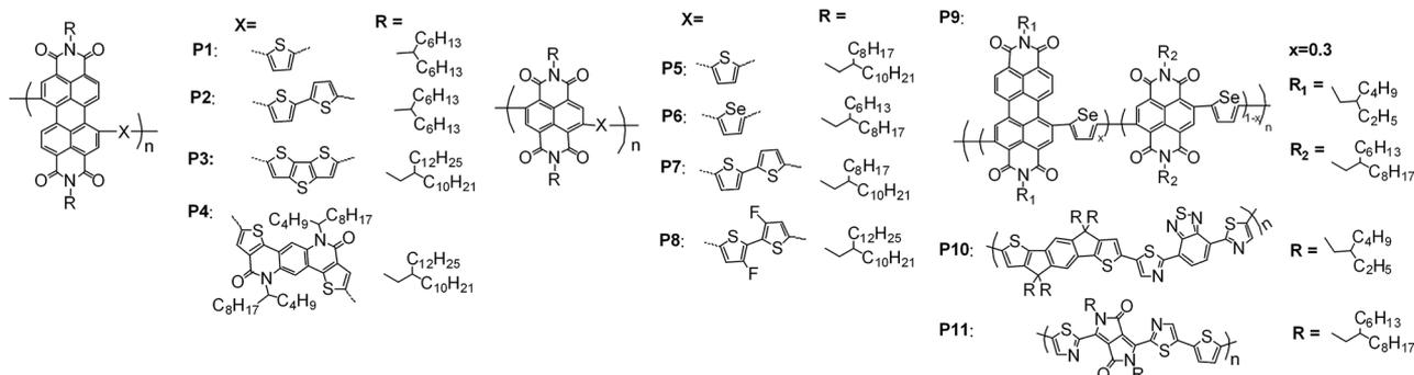
Fig. 15 Chemical structures of the typical reported PDI, NDI and other electron-accepting unit based polymer acceptors.
