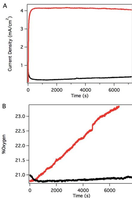
Fig. 4 (A) Controlled potential electrolysis (CPE) of solutions containing **3** (red) and without catalyst (black) at 1.8 V vs. NHE. (B) Headspace O<sub>2</sub> fluorescence detection during CPE of solutions containing **3** (red) and without catalyst (black). Conditions: 0.45 mM catalyst, 0.1 M phosphate at pH 7, 1.4 cm<sup>2</sup> planar ITO electrode.
