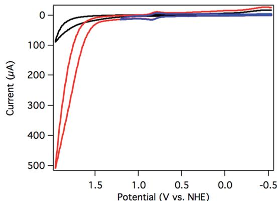
Fig. 3 CV of  $[\text{Ru}(\text{Py}_3\text{PO})(\text{bpy})(\text{OH}_2)_2]^{2+}$  (**3**) swept anodically to 1.95 V (red) and 1.2 V (blue) vs. NHE. A catalyst-free background scan is shown in black. The reduction near  $-0.5$  V is assigned to  $\text{O}_2$  reduction. Conditions:  $250 \text{ mV s}^{-1}$  scan rate, pH 7 0.1 M phosphate buffer, 3 mm glassy carbon disk working electrode, Pt wire counter electrode, Ag/AgCl reference electrode.
