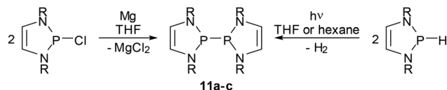
Scheme 12 Syntheses of bis-diazaphospholenyls. Reactions are carried out at ambient temperature (R = tBu ( 11a ), Mes ( 11b ), Dipp ( 11c )).
