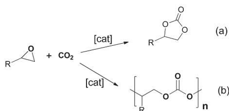
**Scheme 1** (a) Cycloaddition and (b) copolymerization of CO<sub>2</sub> and epoxides.
