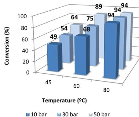
Fig. 4 Effect of CO<sub>2</sub> pressure and temperature on the coupling of 1,2-epoxyhexane and CO<sub>2</sub> using the 1/TBAB catalyst system. Reaction conditions: catalyst 0.2 mol%, TBAB 0.2 mol%, 18 h. Reactions were run in duplicate.
