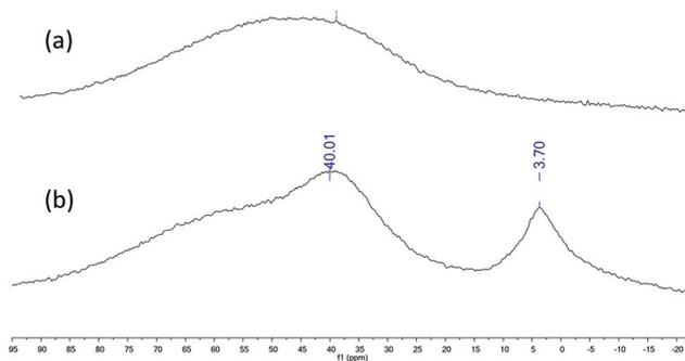
Fig. 7 <sup>27</sup>Al NMR spectra of complex **1** (a) and a mixture **1**/styrene oxide (1 : 1) (b) in CDCl<sub>3</sub>.
