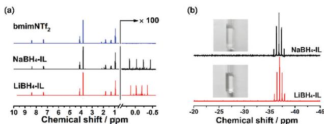
**Fig. 2** (a) <sup>1</sup>H NMR spectra of pristine bmimNTf<sub>2</sub>, NaBH<sub>4</sub>-IL and LiBH<sub>4</sub>-IL samples; (b) <sup>11</sup>B NMR spectra of the NaBH<sub>4</sub>-IL and LiBH<sub>4</sub>-IL samples. The inset pictures are the photographs of the corresponding samples.
