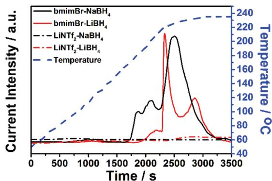
**Fig. 6** TPD curves of bmimBr-NaBH<sub>4</sub> (black, solid), bmimBr-LiBH<sub>4</sub> (red, solid), LiNTf<sub>2</sub>-NaBH<sub>4</sub> (black, dash dot) and LiNTf<sub>2</sub>-LiBH<sub>4</sub> (red, dash dot) samples. The temperature profile is demonstrated as blue dashed line.
