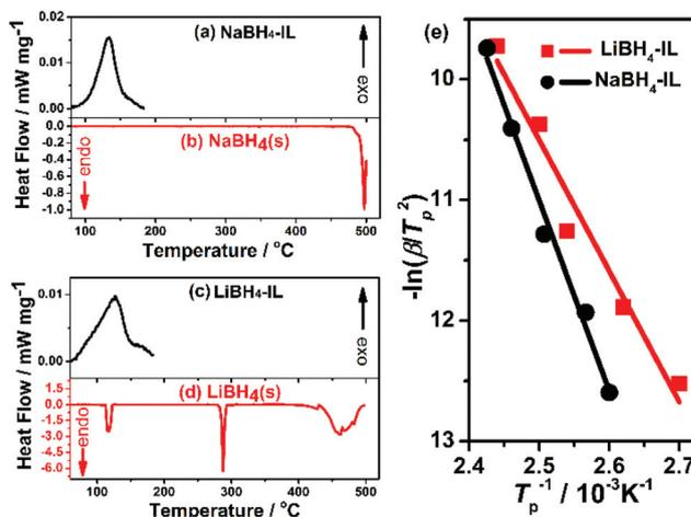
Fig. 5 DSC curves of NaBH<sub>4</sub>-IL and solid state NaBH<sub>4</sub> (a, b) and LiBH<sub>4</sub>-IL and solid state LiBH<sub>4</sub> (c, d) at a heating rate of 2 K min<sup>-1</sup>. The Kissinger's plots of NaBH<sub>4</sub>-IL (black) and LiBH<sub>4</sub>-IL (red) are demonstrated in (e). The apparent activation energy ( $E_a$ ) is calculated from the slope of the fitted lines (the solid lines) according to the Kissinger's equation (eqn (3)).
