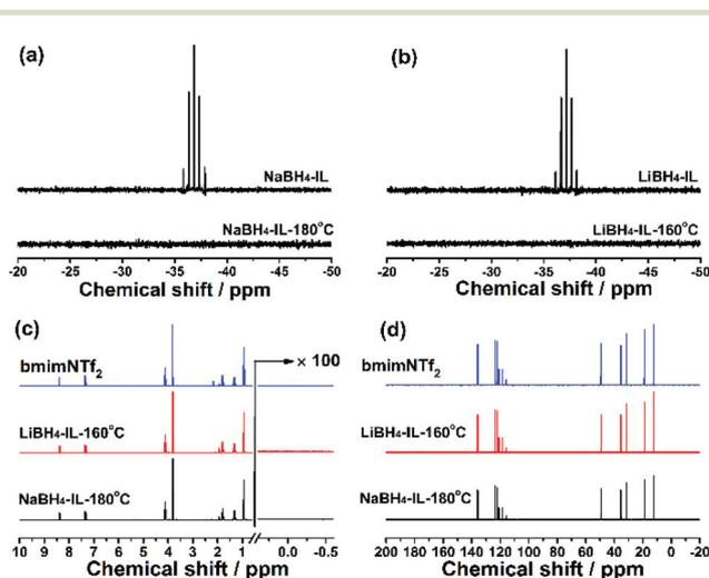
Fig. 4  $^{11}\text{B}$  NMR spectra of the  $\text{NaBH}_4\text{-IL}$  (a) and  $\text{LiBH}_4\text{-IL}$  (b) samples before and after dehydrogenation.  $^1\text{H}$  NMR (c) and  $^{13}\text{C}$  NMR (d) spectra of pristine  $\text{bmimNTf}_2$  and dehydrogenated samples. The  $^{13}\text{C}$  NMR spectra are recorded without deuterated solvents.
