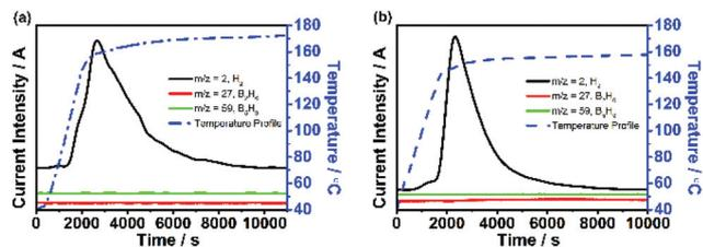
Fig. 7 TPD/MS curves of NaBH<sub>4</sub>-bmmimNTf<sub>2</sub> (a) and LiBH<sub>4</sub>-bmmimNTf<sub>2</sub> (b) samples. The MS signals for H<sub>2</sub> ( $m/z = 2$ , black), B<sub>2</sub>H<sub>6</sub> ( $m/z = 27$ , red), and B<sub>5</sub>H<sub>9</sub> ( $m/z = 59$ , green) are demonstrated in solid lines. The blue dashed lines show the temperature profile of the dehydrogenation reaction.
