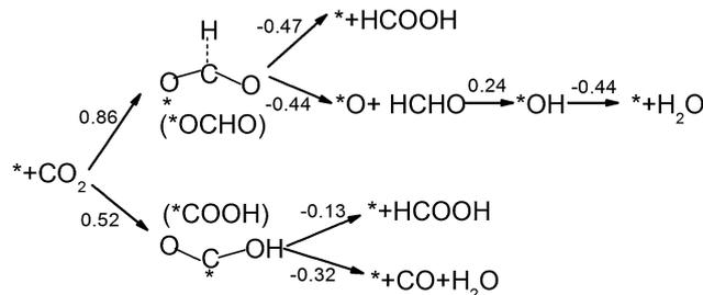
Fig. 5 Free energy variations between intermediates for Edge-2gN graphene catalyst. ( $\text{H}^+(\text{aq}) + \text{e}^-$ ) in each electron step is omitted for simplification. The "\*" represents an active site.
