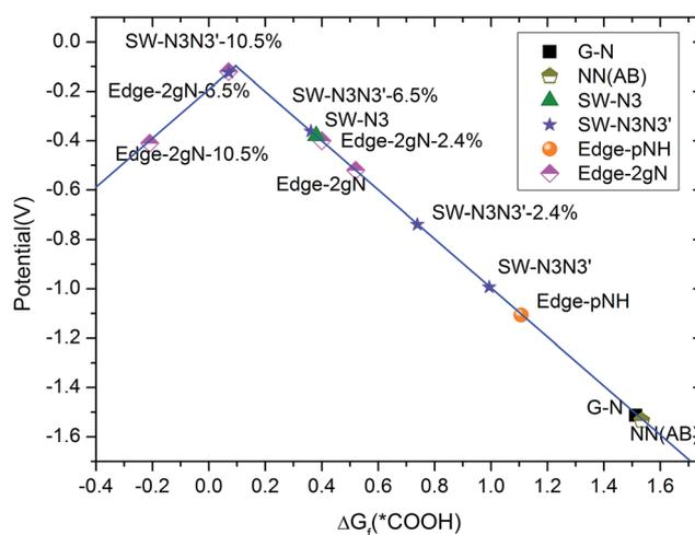
Fig. 7 Calculated limiting potentials for  $CO_2$  to  $CO$  reduction. Curvature is added by reducing the lattice parameter along the X direction (shown in Fig. 2), which is presented by the percentage of lattice parameter reduced.
