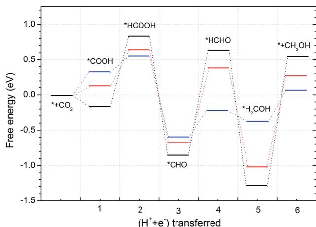
Fig. 8 Free energy variations for CH<sub>3</sub>OH production. The black, red and blue lines correspond to the structures with the lattice parameter reduced for 10.5, 6.5 and 4.0%, respectively.
