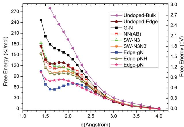
Fig. 3 Free energy profiles of CO<sub>2</sub> approaching C sites with large DOS just below the Fermi level in N doped graphenes for G-N, NN(AB), SW-N3, SW-N3N3', Edge-gN, Edge-pN, Edge-pNH and un-doped bulk surface and edge structures. The approaching distance is that between C atom in CO<sub>2</sub> and the candidate sites in catalysts. The free energy profile for O atom in CO<sub>2</sub> approaching candidate sites are also checked in ESI.†
