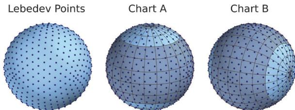
Fig. 17 Locations of the 590 Lebedev quadrature points and the two charts A and B used to deal with singularities at the poles.
