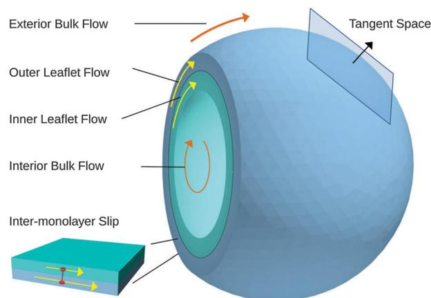
**Fig. 1** Vesicle hydrodynamics. We take into account the hydrodynamics within each leaflet of the bilayer, the intermonolayer slip between leaflets, and the traction stresses for both the solvent fluid trapped interior to the vesicle and the solvent fluid exterior to the vesicle. We use a covariant formulation of the continuum mechanics.
