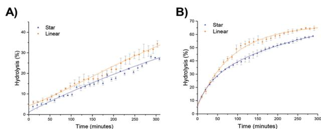
**Fig. 7** Hydrolysis kinetics of 2-20 and the linear analogue PEGA<sub>98</sub>-*b*-(DMAEA<sub>60</sub>-*co*-MA<sub>13</sub>) at (a) 25 °C and (b) 50 °C, in D<sub>2</sub>O as determined by <sup>1</sup>H NMR spectroscopy. Error bars produced from the standard deviation of 3 repeats.
