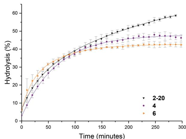
Fig. 6 Hydrolysis kinetics of short, medium and long armed PEGA stars (2-20, 4, and 6 respectively), at 50 °C in D<sub>2</sub>O as determined by <sup>1</sup>H NMR spectroscopy. Error bars produced from the standard deviation of 3 repeats.
