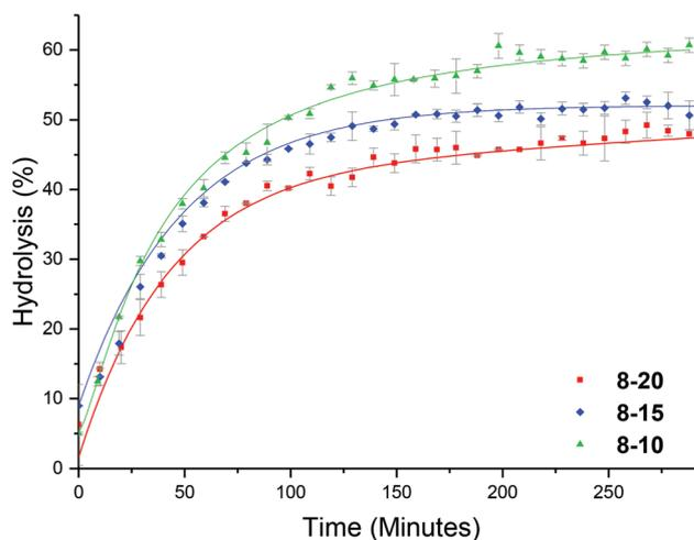
**Fig. 8** Hydrolysis kinetics of PHEA-*b*-(DMAEA-*co*-DEGDA) of varying crosslinking densities, in D<sub>2</sub>O at 50 °C as determined by <sup>1</sup>H NMR spectroscopy. Error bars produced from the standard deviation of 3 repeats.
