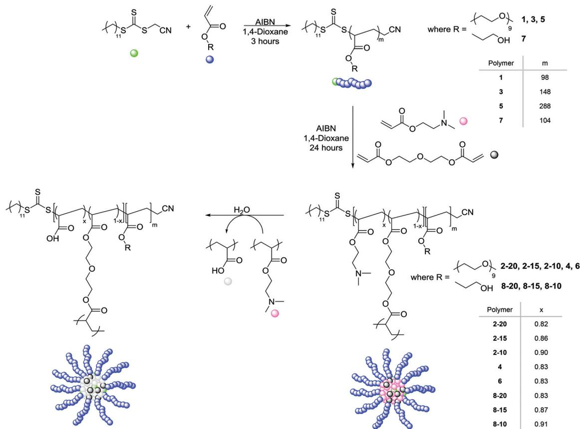
**Scheme 1** Synthesis of DMAEA functionalized polymeric stars (2-20, 2-15, 2-10, 4, 6, 8-20, 8-15 and 8-10) via an arm-first approach using RAFT polymerization, and hydrolysis of the amine functionality to acrylic acid moieties. Amine content determined by the polymer DPs calculated using  $^1\text{H}$  NMR spectroscopy.
