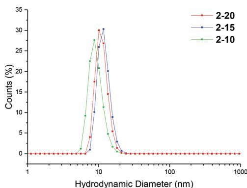
**Fig. 2** Size distributions, by number, for PEGA armed particles 2-20, 2-15, 2-10, obtained by DLS (detection angle = 173°) at 5 mg mL<sup>-1</sup> carried out in chloroform at 25 °C.
