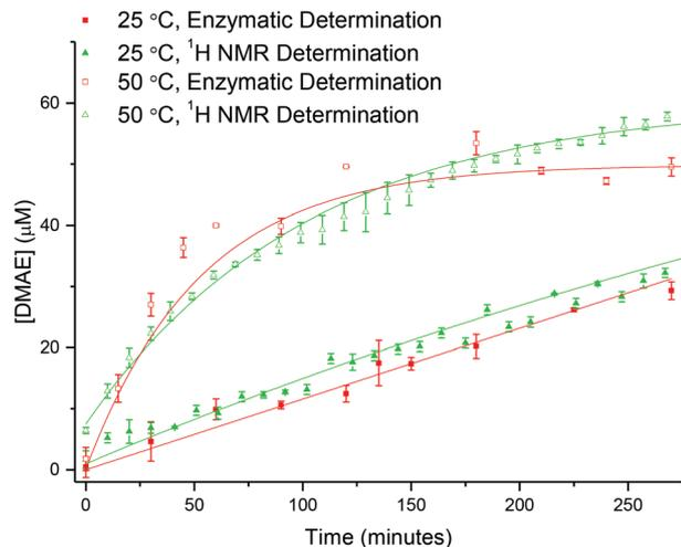
**Fig. 10** Comparison between the theoretical concentration of DMAE released based on  $^1\text{H}$  NMR spectroscopic analysis (green) and enzymatically determined (red) at 25 and 50 °C. Error bars produced from the standard deviation of three repeats.
