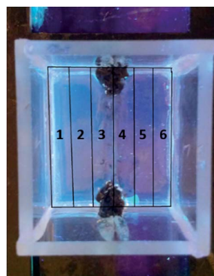
Fig. 4 Division of the diffusion cell into 6 regions for purposes of sampling.
