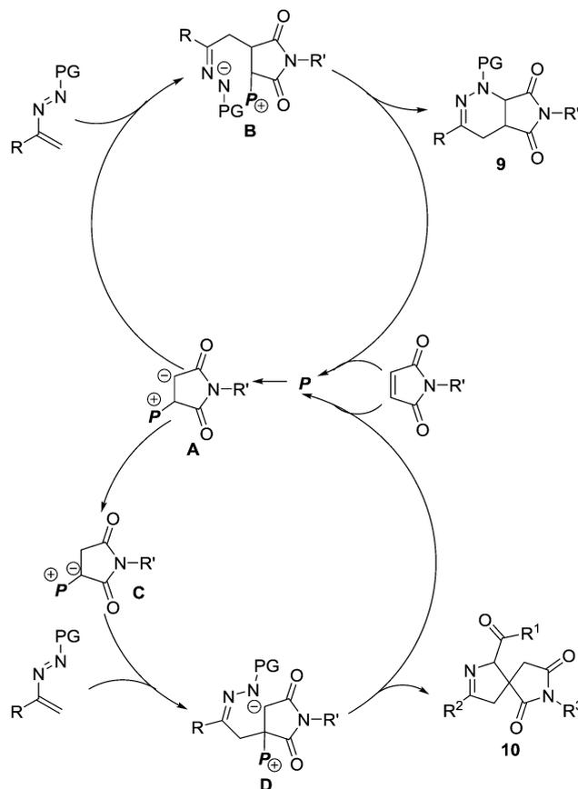
Scheme 5 Proposed mechanism for the PPh<sub>3</sub>-mediated formal [4+1]/[4+2] annulation of maleimides with *in situ* generated azoalkenes.
