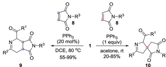
Scheme 4 PPh<sub>3</sub>-Mediated formal [4+1]/[4+2] annulation of maleimide with *in situ* generated azoalkenes.
