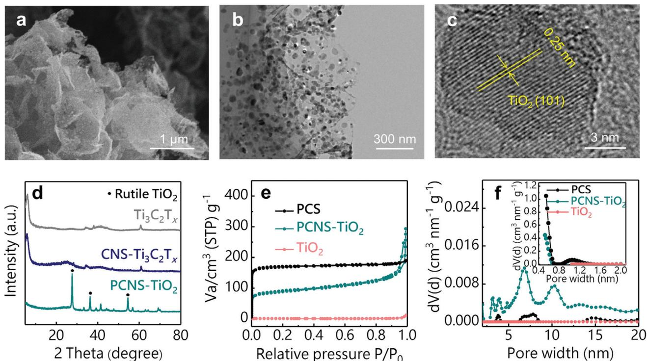
**Fig. 2** (a) SEM, (b) TEM and (c) HRTEM images of PCNS-TiO<sub>2</sub>. (d) XRD patterns of Ti<sub>3</sub>C<sub>2</sub>T<sub>x</sub>, CNS-Ti<sub>3</sub>C<sub>2</sub>T<sub>x</sub> and PCNS-TiO<sub>2</sub>. (e) N<sub>2</sub> adsorption–desorption isotherms and (f) pore size distributions of the PCS, PCNS-TiO<sub>2</sub> and TiO<sub>2</sub>.
