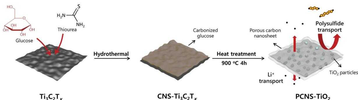
Fig. 1 Scheme of the preparation process of PCNS-TiO<sub>2</sub>.
