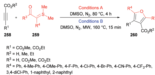
Scheme 67 Regiospecific synthesis of polysubstituted furans from sulfonium acylmethylides and acetylenic esters.
