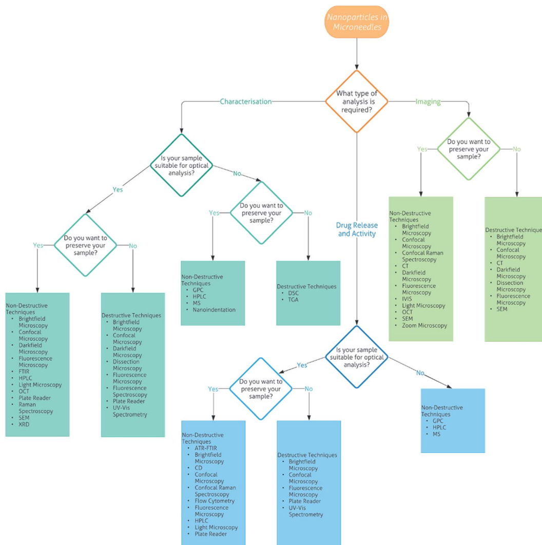
Fig. 7 Flowchart of the analytical techniques that can be used for the characterisation, imaging and drug release and activity of nanoparticles in microneedles.
