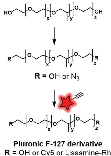
Fig. 28 Fluorescent labeling of Pluronic F-127 with Cy5 and Lissamine-Rh by click chemistry described by Reisch and coworkers.
