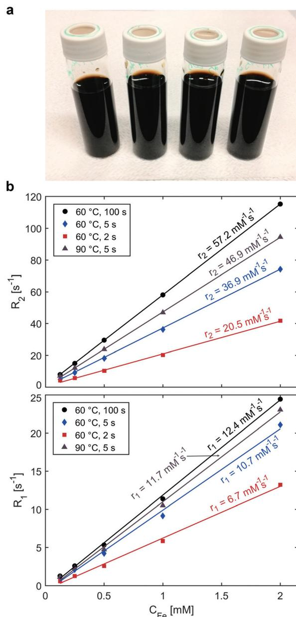
**Fig. 5** (a) IONP solutions synthesised with quenching times of 100, 5 and 2 s at 60 °C and 5 s at 90 °C (from left to right) selected for MRI contrast performance evaluation. (b) Relaxation rates  $R_2$  (transversal, top) and  $R_1$  (longitudinal, bottom) vs. iron concentration in the (consecutively diluted) dialysed samples ( $C_{\text{Fe}}$ ) to determine  $r_1$  and  $r_2$  (*i.e.*, the slope) for IONPs synthesised at co-precipitation temperatures and quenching times as indicated.
