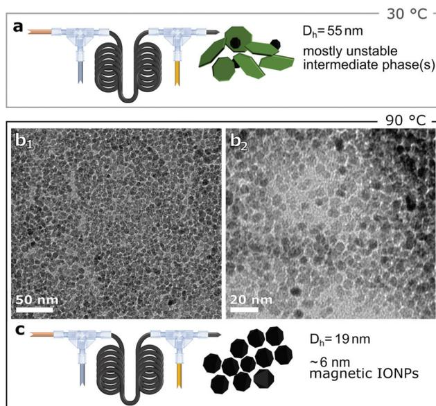
Fig. 4 (a) Schematic of flow synthesis with co-precipitation performed at 30 °C. (b<sub>1–2</sub>) TEM images of IONPs synthesised with co-precipitation performed at 90 °C,  $D_{\text{TEM}} = 6.1 \pm 0.9$  nm. (c) Schematic of flow synthesis with co-precipitation initiated at 90 °C. Fig. S5† shows the particle size distribution. For both temperatures, quenching was performed at 5 s.
