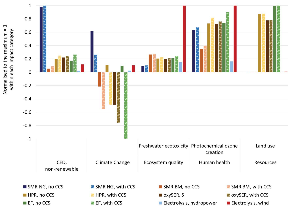
Fig. 10 Performance of selected individual hydrogen producing technologies in selected impact categories per MJ of hydrogen. Scores are normalised to 1, which corresponds to the maximum score in each impact category, i.e. the technology which performs worst on the positive scale or, in the case of climate change, best on the negative scale.
