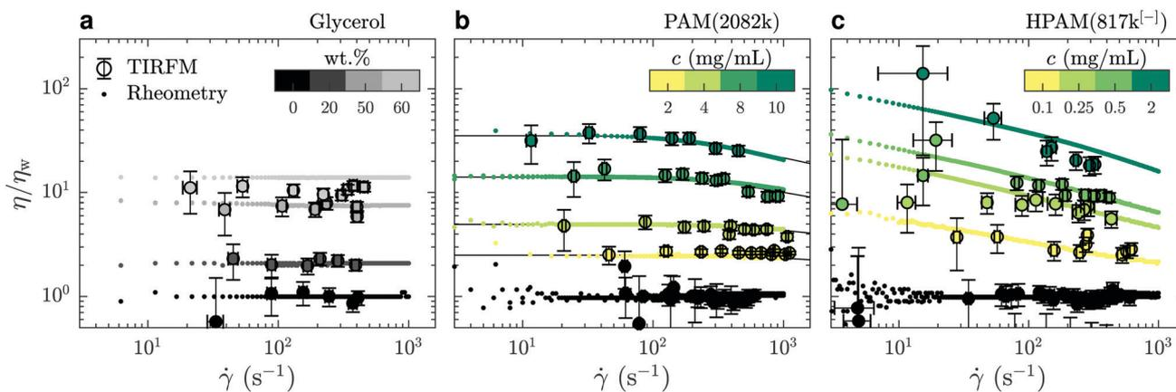
**Fig. 3** Comparison of the mechanical behaviours of: (a) water/glycerol mixtures; (b) PAM(2082k) solutions; and (c) HPAM(817k<sup>-1</sup>) solutions. TIRFM velocimetry data are plotted in circles and rotational rheometry data are plotted using dots; black lines in panel (b) indicate predictions of the universal model of ref. 34. The color bars indicate the concentration of each solution and water is always represented in black. All the data shown here were collected without added salt.
