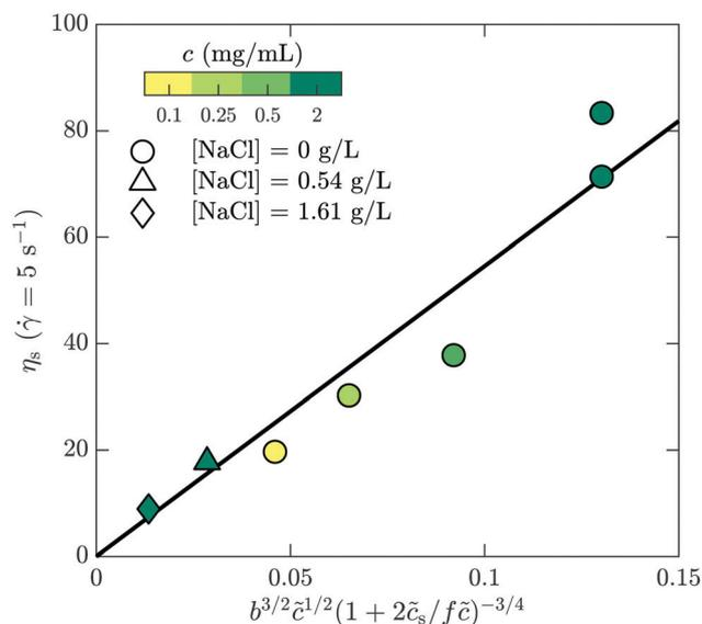
Fig. 7 Bulk rheology measurements of the steady-shear viscosity for HPAM(817k<sup>L-1</sup>) at a shear rate of 5 s<sup>-1</sup>, as a function of the scaling variable developed by Dobrynin and coworkers.<sup>41</sup>
