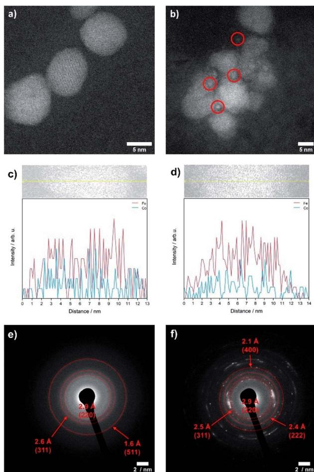
Fig. 7 TEM images of  $\text{CoFe}_2\text{O}_4$  ( $x = 1$ ) nanoparticles before (a) and after OER (b), TEM-EDX line scans on a single particle for  $\text{CoFe}_2\text{O}_4$  ( $x = 1$ ) before (c) and after electrochemical treatment (d) and SAED patterns after OER measurements for  $\text{Co}_x\text{Fe}_{3-x}\text{O}_4$  with  $x = 2.25$  (e) and 2.50 (f).
