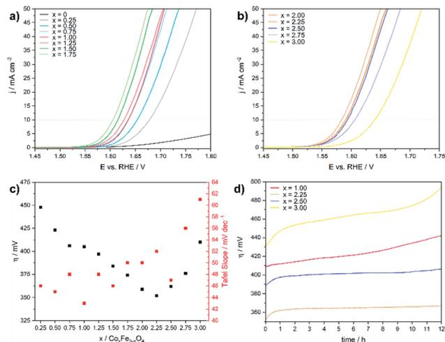
Fig. 4 Linear sweep voltammograms for (a)  $\text{Co}_x\text{Fe}_{3-x}\text{O}_4$  ( $x = 0-1.75$ ) and (b)  $(\text{Co}_{x/3}\text{Fe}_{(1-x)/3})\text{O}$  ( $x \geq 2$ ) in 1 M KOH electrolyte with a scan rate of  $5 \text{ mV s}^{-1}$ , (c) overpotential and Tafel slope versus the cobalt content and (d) chronoamperometry measurements at  $10 \text{ mA cm}^{-2}$  (geometrical surface area).
