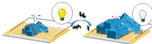
Fig. 5 Switchable MIL-53-carbon additive composite for CO 2 sensing. 25
