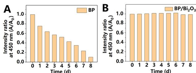
Fig. 4 Variations in the absorption intensity ratio at 450 nm of BP (A) and BP/Bi<sub>2</sub>O<sub>3</sub> heterostructures (B) after standing in water for different durations of time. Adapted and modified with permission from ref. 26 Copyright (2018) Elsevier.
