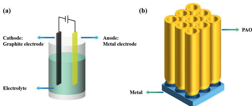
Fig. 1 (a) Anodizing device; (b) PAO array.
