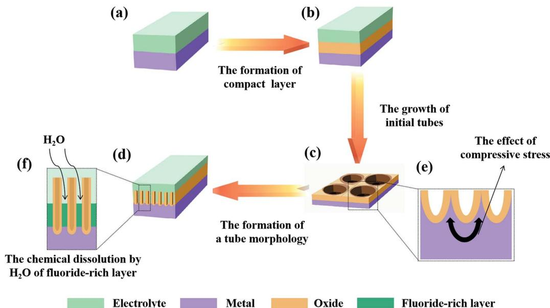
Fig. 3 Schematic of the mechanism of self-organization theory.
