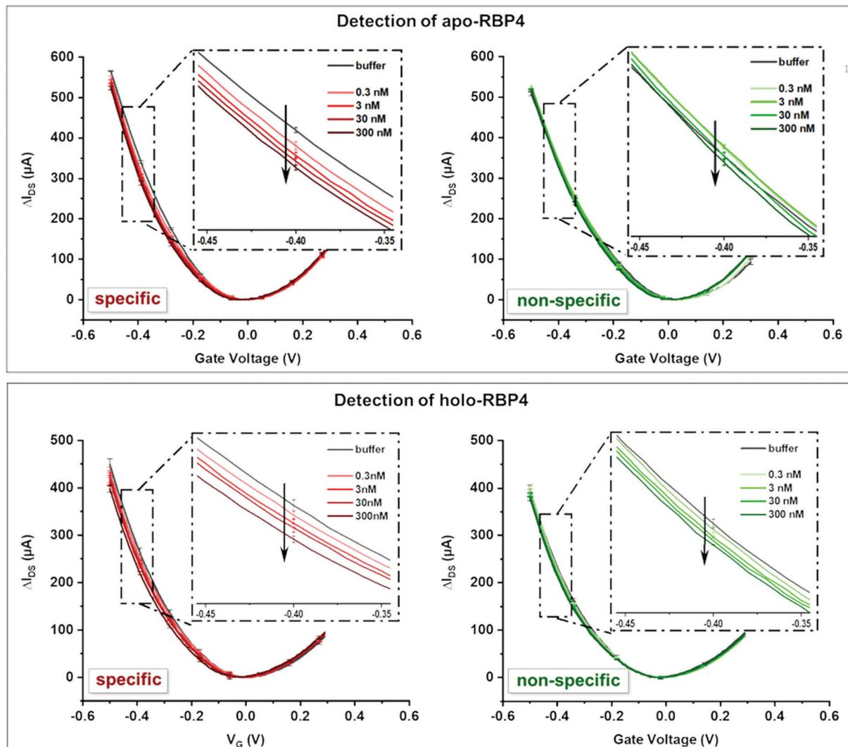
Fig. 3 Top: Detection of apo-RBP4. Bottom: Detection of holo-RBP4.  $I_D V_G$  curves are an average of a minimum of 3 individual curves with error bars showing the standard deviation. Both devices showed significantly more pronounced shifts in their  $I_D V_G$  characteristics upon specific analyte binding.
