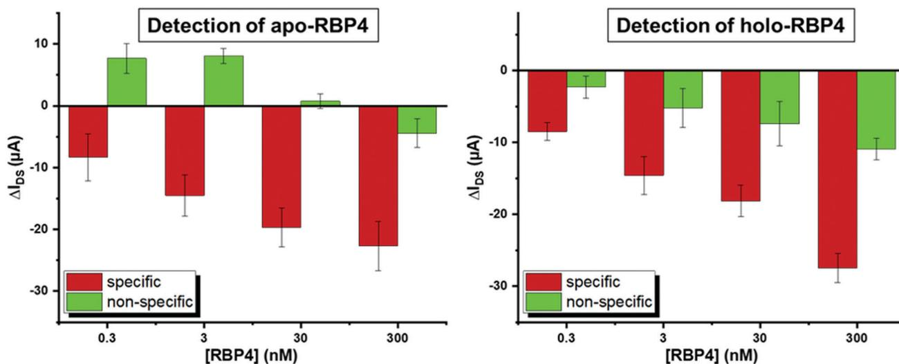
Fig. 4 Average difference in current at  $-0.4$  V upon addition of increasing concentrations of RBP4.  $\Delta$ -Values shown are averages of a minimum of three independent experiments on different devices. Error bars show the standard deviation.
