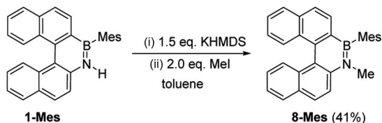
Scheme 5 Synthesis of 8-Mes by functionalizing 1-Mes.
