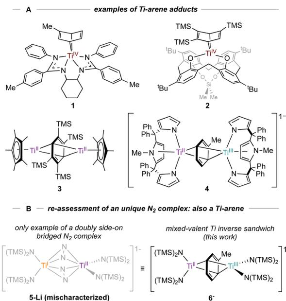
**Fig. 1** A: Examples of monometallic (1–2) and bimetallic coordinated arenes (3–4). B: New examples of inverse sandwich toluene complexes (6-K and 6-Li) indicate that a reported Ti<sub>2</sub>–(N<sub>2</sub>)<sub>2</sub> complex 5-Li was originally mischaracterized.<sup>26</sup> Counteranions omitted for clarity.
