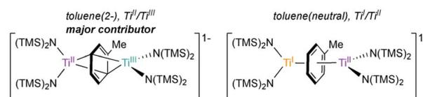
**Fig. 3** Electronic representation of **6-K** as either Ti<sup>II</sup>/Ti<sup>III</sup> bridged by a toluene dianion (left) or Ti<sup>I</sup>/Ti<sup>II</sup> bridged by a neutral toluene (right).
