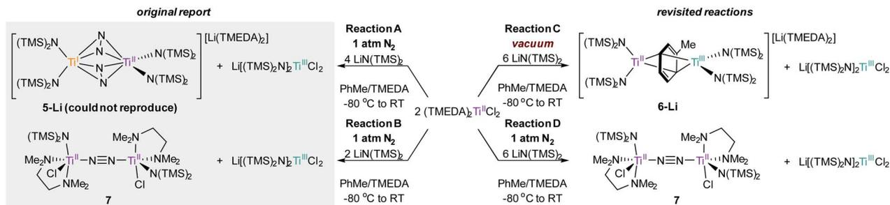
Fig. 8 Previously reported conditions for the synthesis of 5-Li and 7 (left) and the re-examined reactivity of  $(\text{TMEDA})_2\text{TiCl}_2$  toward  $\text{N}_2$  and in vacuum conditions for the synthesis of 6-Li and 7 (right).
