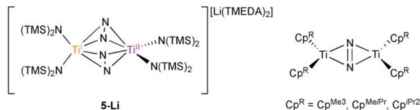
Fig. 4 Reported examples of bimetallic Ti complexes bridged by a side-on  $\text{N}_2$  ligand. Left: double side-on  $\text{Ti}-(\text{N}_2)_2\text{-Ti}$ , **5-Li**, complex.<sup>26</sup> Right: single side-on  $\text{N}_2$  titanocene complexes.<sup>5,7</sup>
