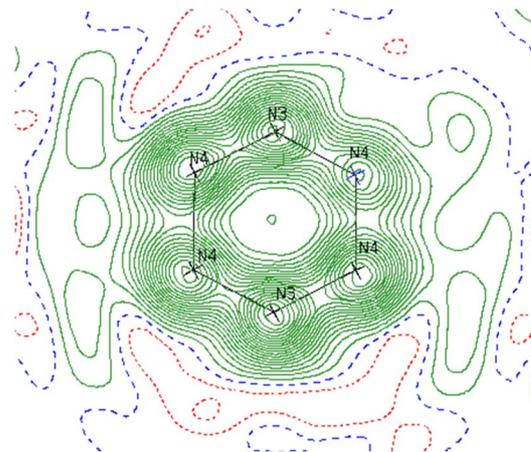
Fig. 6 Contour map of  $F_{\text{obs}}$  for **5-Li** showing the plane bisecting the  $\text{Ti-Ti}$  vector. Range:  $-0.60$  to  $3.80 \text{ e}^- \text{ \AA}^{-3}$  in steps of  $0.20$ . Negative contours are shown in red and positive in green. Residual electron density outside of the N ring indicates likely partial occupancy of another atom at those positions.
