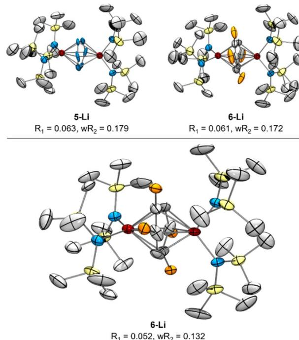
Fig. 7 Top: re-solved SC-XRD of reported **5-Li** reflection data as either **5-Li** (left) or **6-Li** (right) as possible solutions, with displacement ellipsoids drawn at the 50% probability level. Bottom: XRD from new reflection data of re-synthesized **6-Li** following Reaction C from Fig. 8. Orange ellipsoids are disordered Me groups of the toluene dianion in 4 positions. Hydrogen atoms,  $\text{NTMS}_2$  disorder, and counterions were removed for clarity.
