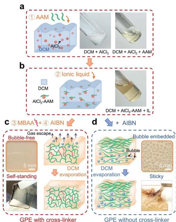
**Fig. 1** Preparation schematic of the gel polymer electrolyte (GPE). (a) The complexation of the AAM monomer with  $\text{AlCl}_3$  in DCM solvent. (b) Introducing abundant ionic liquid (IL). (c) The GPE polymerized with an MBAA cross-linker delivering a bubble-free and self-support membrane. (d) Typical fabrication showing a sticky GPE with bubbles.
