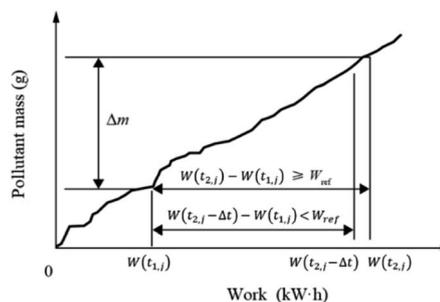
Fig. 7 Schematic diagram of the work-based window method.
