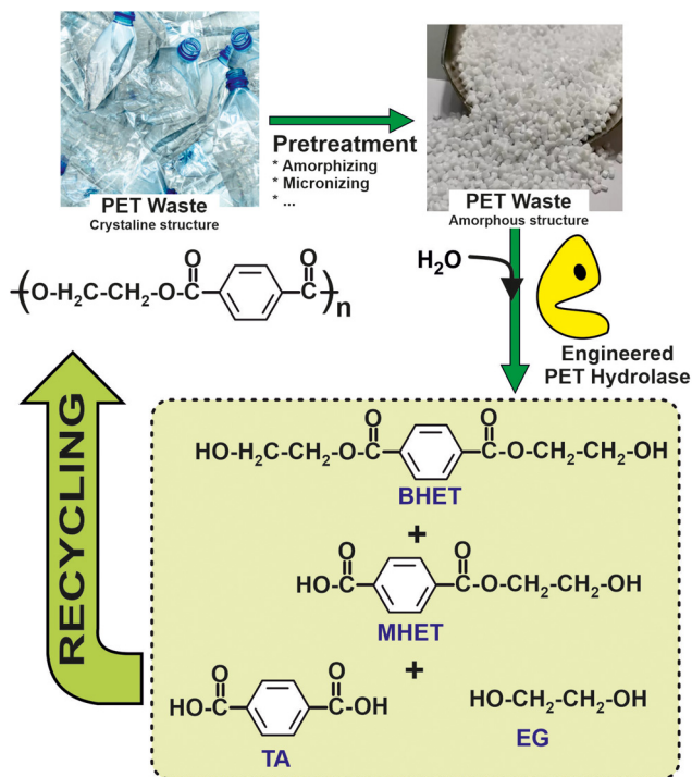
Fig. 8 Schematic representation of a circular chemistry process for recovery and reuse of polyethyleneterephthalate (PET), based on the enzymatic hydrolysis by means of engineered biocatalysts. 105
