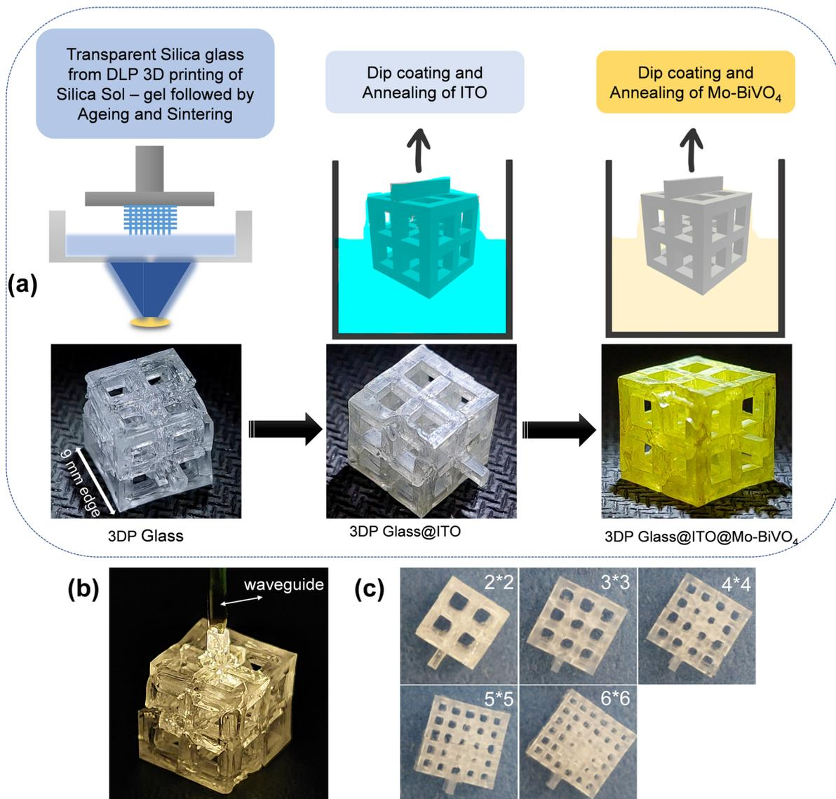
**Fig. 1** (a) Illustration of the fabrication of semi-transparent 3D lattice structures for photoelectrochemical water oxidation. (b) Picture of the 3D printed glass in a dark room with a light waveguide joined at the tip of the lattice to demonstrate waveguiding of the light through the lattice structure. (c) Picture of the 3D printed glass lattice structures with varying degrees of porosity; all the printed lattices have the dimension of a 9 mm × 9 mm × 9 mm cube.
