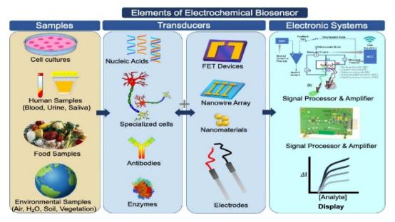
Fig. 4 Illustration of the design elements of biosensors used to detect target test samples, with an emphasis on the electrochemical bio-sensing platforms, which translate biochemical data into current or voltage signals on the surface of an electrochemical biosensor. This figure has been adapted/reproduced from ref. 23 with permission from Elsevier, copyright 2021.
