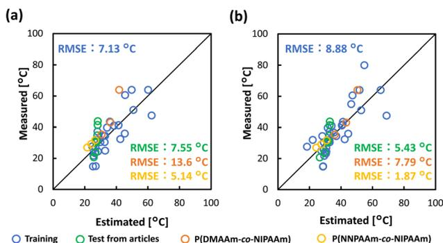
Fig. 5 The relationship between estimated  $T_{CP}$ s from prediction model and measured values: (a) Compared by prediction model of eqn (1). (b) Compared by prediction model of eqn (2) with corrected coefficients.
