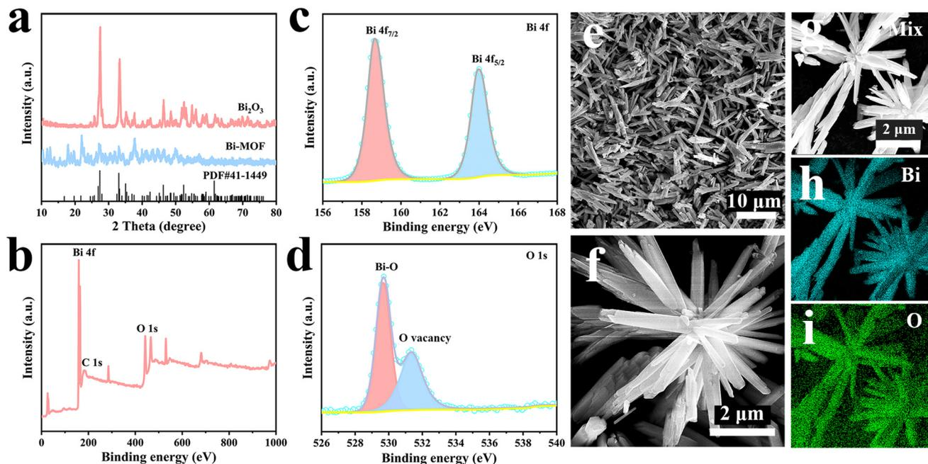
Fig. 5 (a) XRD patterns of Bi-MOF and  $\text{Bi}_2\text{O}_3$ . (b) XPS survey of  $\text{Bi}_2\text{O}_3$ . (c and d) XPS spectrum of Bi 4f and O 1s of  $\text{Bi}_2\text{O}_3$ . (e and f) SEM images of  $\text{Bi}_2\text{O}_3$ . (g-i) EDS mapping of  $\text{Bi}_2\text{O}_3$ .
