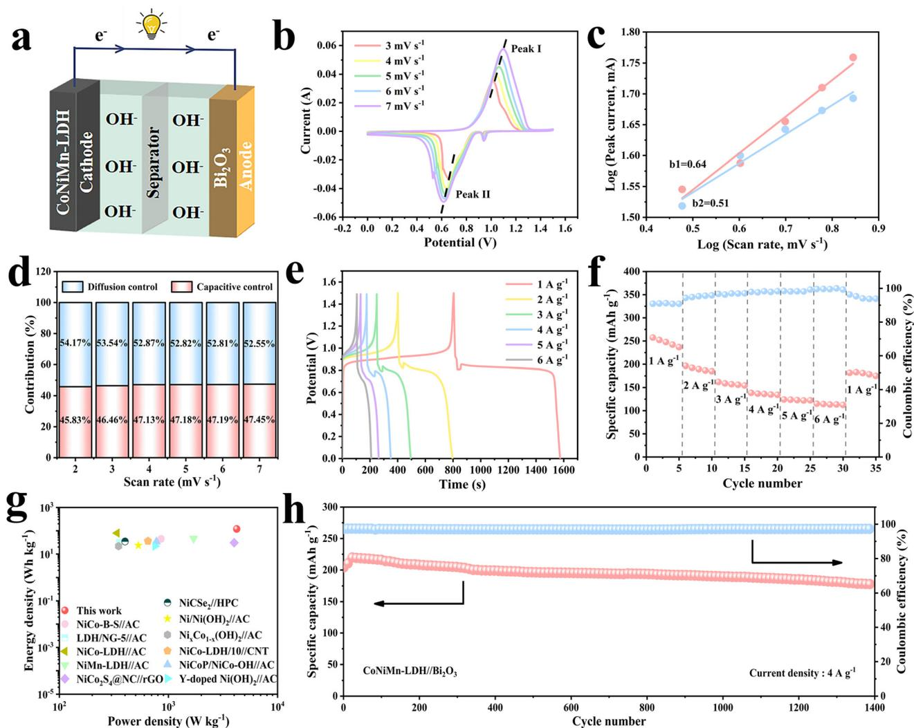
**Fig. 7** (a) Schematic illustration of the CoNiMn-LDH//Bi<sub>2</sub>O<sub>3</sub> alkaline battery. (b) CV curves. (c) Plots of  $\log(i)$  versus  $\log(v)$ . (d) Capacitance contribution. (e) GCD curves. (f) Rate performance. (g) Ragone plots. (h) Cycling performance.
