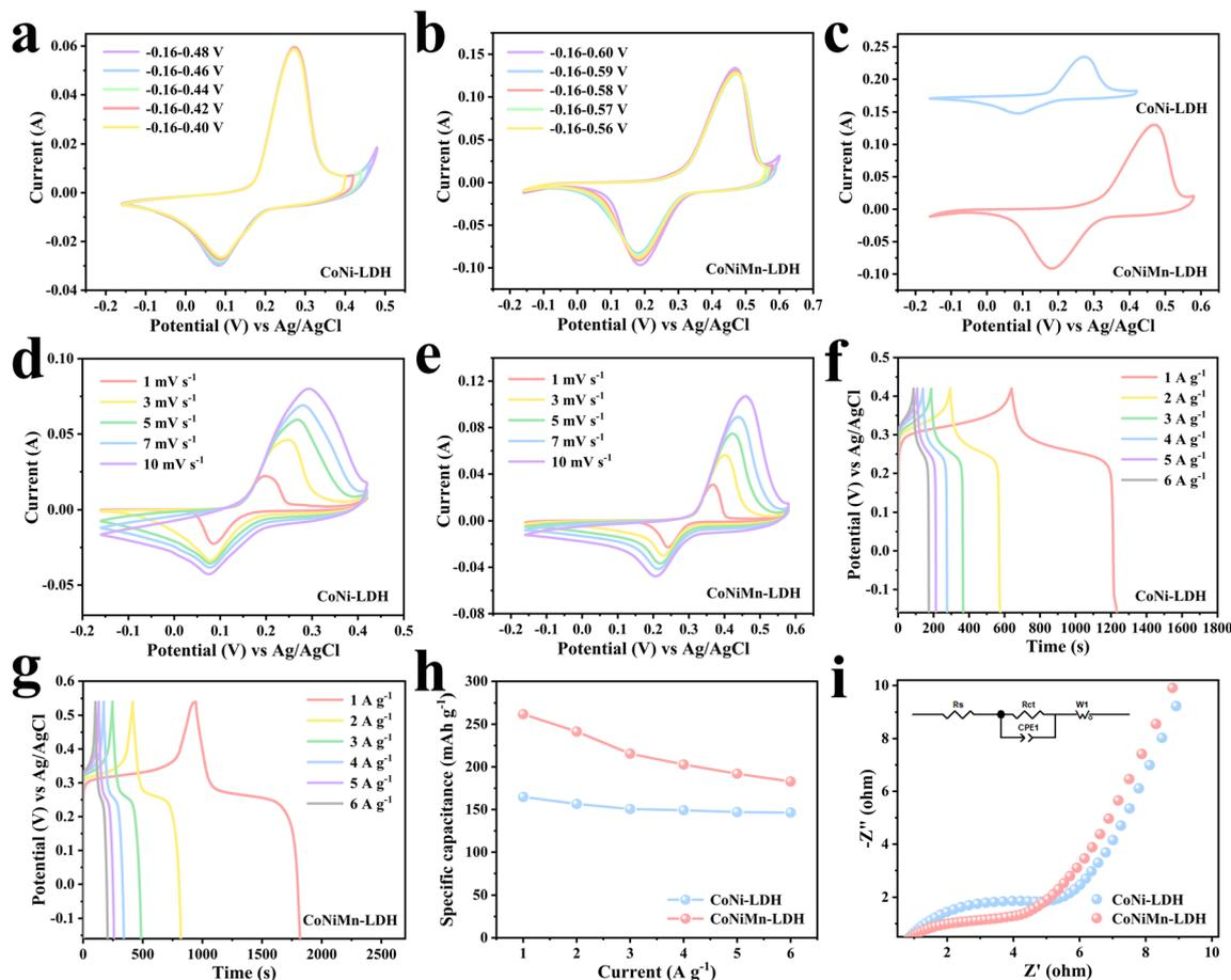
**Fig. 4** (a and b) CV curves of CoNi-LDH and CoNiMn-LDH at  $10 \text{ mV s}^{-1}$ . (c) Optimal voltage windows. (d and e) CV curves at different scan rates. (f and g) GCD curves. (h) Specific capacity. (i) Nyquist plots.
