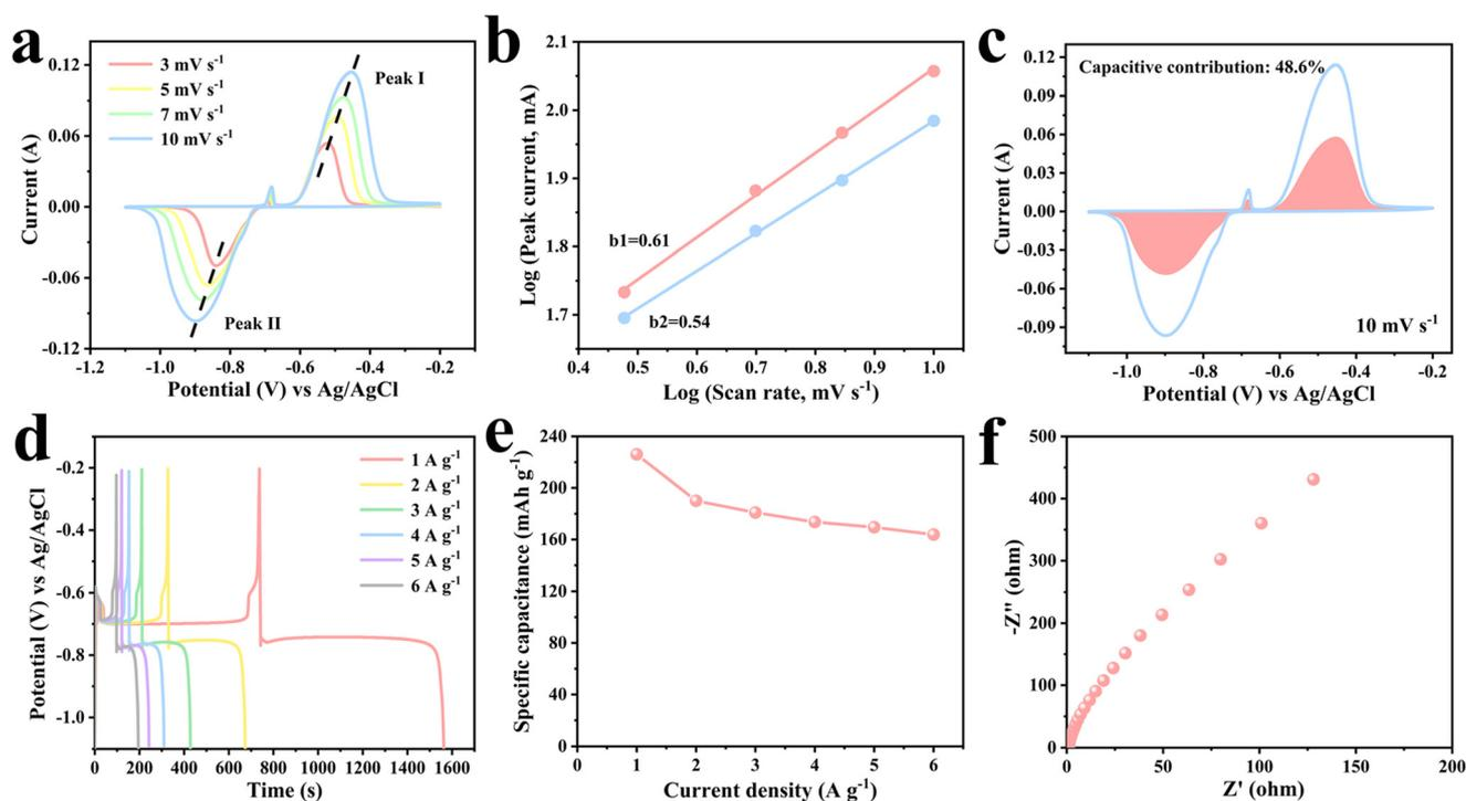
Fig. 6 Electrochemical performance of  $\text{Bi}_2\text{O}_3$ . (a) CV curves at different scan rates. (b) Plots of  $\log(i)$  versus  $\log(v)$ . (c) Capacitive contribution. (d) GCD curves. (e) Specific capacity. (f) Nyquist plots.
