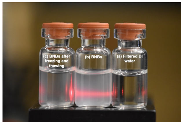
Fig. 3 Tyndall effect test. This image is taken 1 day after making BNBs. We shoot a red laser beam from the right side of the image to the left. (a) The vial containing DI water does not scatter the light as there are no particles inside the sample. (b) The sample containing the BNB solution scatters the laser light due to the presence of BNBs suspended in the vial. (c) This image shows a BNB sample after freezing for 24 \text{ h} and thawing. The degree of scattered light in the thawed BNB solution is considerably reduced compared to the BNB vial without freezing–thawing. This is likely due to the rupture of BNBs during the freezing–thawing process. 14 Both BNB suspensions in (b) and (c) are made by first generating MBs with D_i = 7.0 \mu\text{m} , with 0.17 \text{ wt\% C}_3\text{F}_8 gas, and a lipid solution concentration of 0.50 \text{ mg mL}^{-1} .
