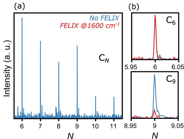
Fig. 2 Representative mass spectrum of C<sub>N</sub> clusters ionized by 118 nm laser light, produced by the desorption and fragmentation of C<sub>60</sub> molecules. Left panel: No FELIX excitation. Right panel: Comparison of intensities without (blue) and with (red) FELIX irradiation at 1600 cm<sup>-1</sup> for C<sub>6</sub> (top) and C<sub>9</sub> (bottom).
