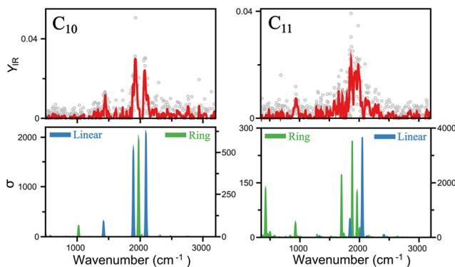
Fig. 4 Comparison of the infrared spectra of linear and ring isomers of  $C_{10}$  and  $C_{11}$ . The top panels depict the experimental data. In the bottom panels, the computed spectra of both isomers is shown. Note different left and right y-axis, as highlighted by the position of the legends. Linear isomers have higher infrared intensities.
