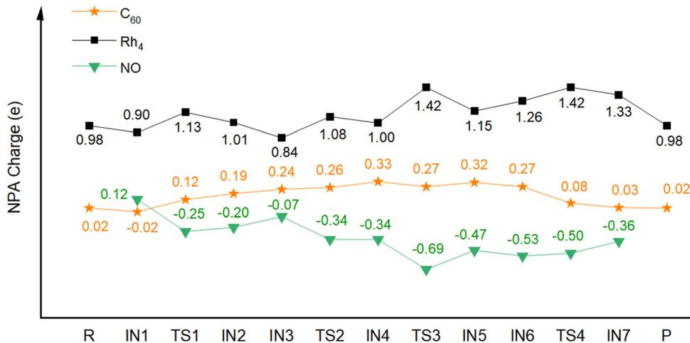
Fig. 3 Calculated NBO partial charges (e) of the Rh<sub>4</sub><sup>+</sup> cluster (black square) and C<sub>60</sub> (orange star) of NO reduction catalyzed by C<sub>60</sub>Rh<sub>4</sub><sup>+</sup>.
