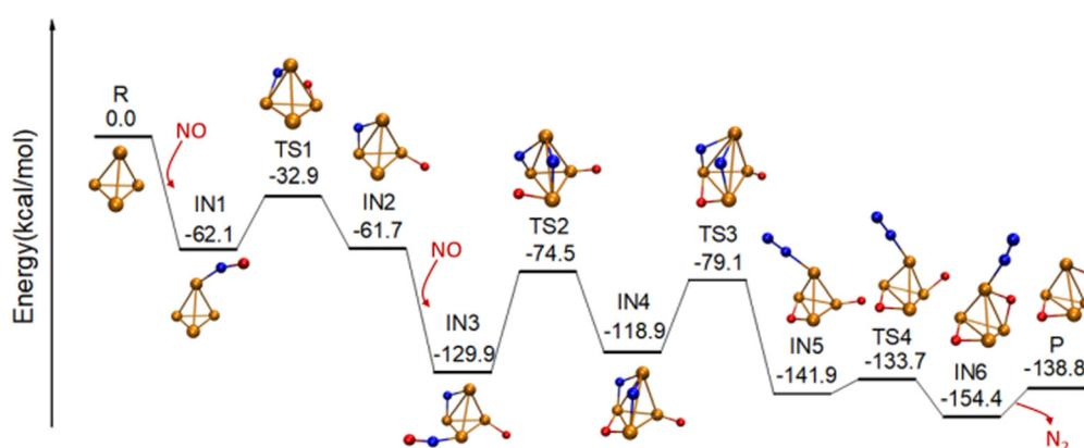
Fig. 2 Reaction pathway of NO reduction on  $Rh_4^+$  calculated at the BPW91/6-31G(d)θSDD level of theory. R stands for reactants, IN for intermediates, TS for transition states, and P for products. All energies are provided relative to the energies of the reactants, *i.e.*,  $Rh_4^+$  and two NO molecules.
