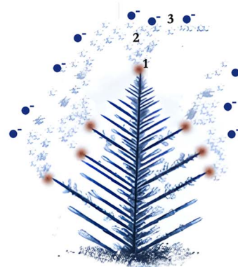
Scheme of ion emission from ice structure
