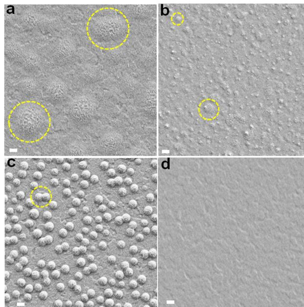
Fig. 2 SEM images ITO/ $\text{bl-TiO}_2$  substrates after spin-coating DMF/DMSO dispersions ( $3.0$   $\text{mg g}^{-1}$ ) of (a) NG-60, (b) NG-100 and (c) NG-200 particles. An SEM of the bare ITO/ $\text{bl-TiO}_2$  substrate is shown in (d) for comparison. The yellow circles highlight coalesced nanogels. Scale bars:  $200$  nm.
