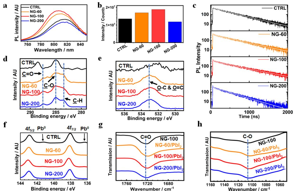
Fig. 5 (a) PL spectra for various perovskite/nanogel systems. (b) The maximum PL intensity from the spectra in (a). (c) TRPL data for various perovskite films. (d) C 1s, (e) O 1s and (f) Pb 4f core level spectra from XPS measurements for the control perovskite and films prepared with nanogels (3 mg g<sup>-1</sup>). (g) C=O and (h) C–O stretching regions of the FTIR spectra measured for NG-100 and the various nanogels mixed with PbI<sub>2</sub>.
