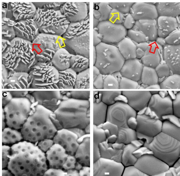
**Fig. 3** Top view SEM images of the perovskite films prepared using (a) NG-60, (b) NG-100, (c) NG-200 and (d) the control without nanogels. The yellow arrows highlight nanofilm bridges between perovskite grains. The red arrows highlight small pinholes in the bridging nanofilms at the junction of three perovskite grains. Scale bars: 200 nm. See also Fig. S11 (ESI<sup>†</sup>).
