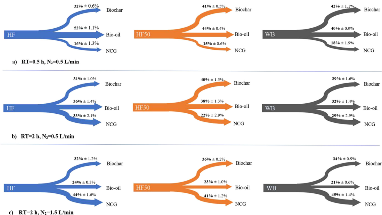
Fig. 8 Distribution of carbon flows to biochar, bio-oil and non-condensable gas (NCG) streams expressed as the % of the total carbon content in the feedstock (for HF, HF50 and WB) (pyrolysis experiments at 550 °C). Results for different combinations of retention time (RT) and N 2 gas flow rate: (a) RT = 0.5 h, N 2 = 0.5 L min -1 ; (b) RT = 2 h, N 2 = 0.5 L min -1 ; and (c) RT = 2 h, N 2 = 1.5 L min -1 . The reported values are calculated based on eqn (1)–(3), following total C analysis on a CHNS elemental analyser (see section 2.4).
