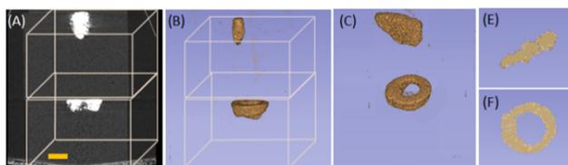
**Fig. 6** (A–C) 3D reconstructions of the micro-CT scans of a stack of two PEGDA-foam composites (bottom: ring, top: post) (lines show a perimeter of each foam); (E and F) cross-sectional images of the ring and post. Scale bar = 1 cm.
