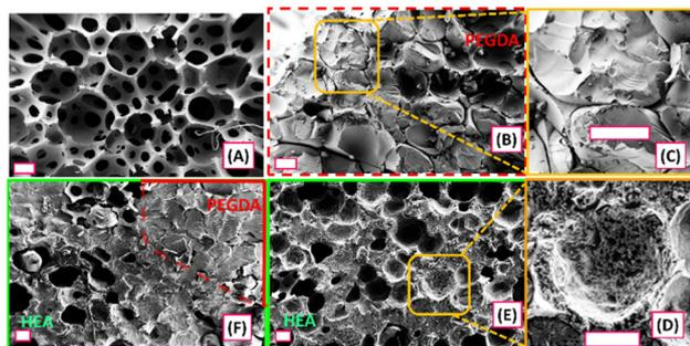
**Fig. 7** SEM cross-sectional images of (A) foam without resin, (B and C) cured PEGDA in foam and zoomed-in images of the selected area, (E and D) cured HEA in foam and zoom-in images of the selected area, and (F) layers of cured PEGDA and HEA in foam. Scale bars = 300  $\mu\text{m}$ .
