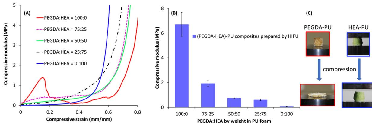
**Fig. 10** (A) Uniaxial compression tests on composites made from foams with PEGDA, HEA, and mixtures of PEGDA and HEA, (B) compressive modulus data of the composites at different weight fractions of PEGDA and HEA (see Table S3†), (C) pictures showing PEGDA-foam and HEA-foam composites before and after compression.
