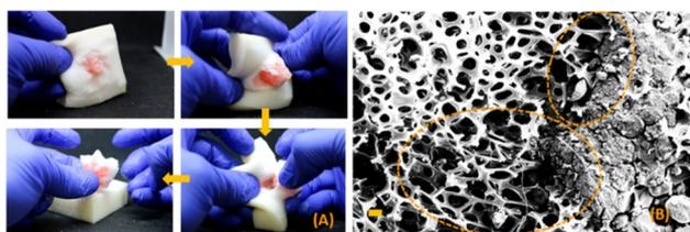
**Fig. 8** (A) Pictures of a cylinder of cured PEGDA in foam while tearing the cured domain from the foam, and (B) SEM image showing intersections between empty foam domains and cured PEGDA-foam composite while under static tension (encircled regions highlight strained foam components). Scale bar = 300  $\mu\text{m}$ .
