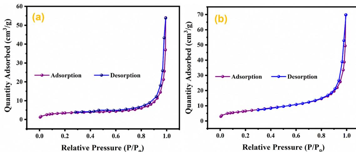
Fig. 9 BET isotherms of (a)  $\text{MnO}_2$ , (b)  $\text{Ag}_{0.05}\text{MnO}_2$ .
