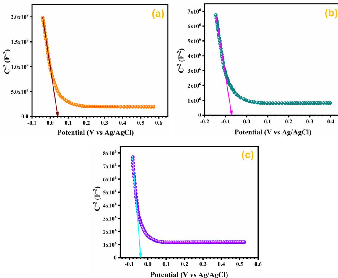
Fig. 12 M-S profile of (a) MnO<sub>2</sub>, (b) Ag<sub>0.05</sub>MnO<sub>2</sub>, and (c) Ag<sub>0.15</sub>MnO<sub>2</sub>.
