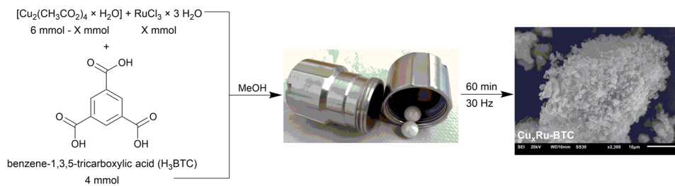
Fig. 1 Schematic representation of the synthesis of the mixed-metal Cu x Ru-BTC MOFs.
