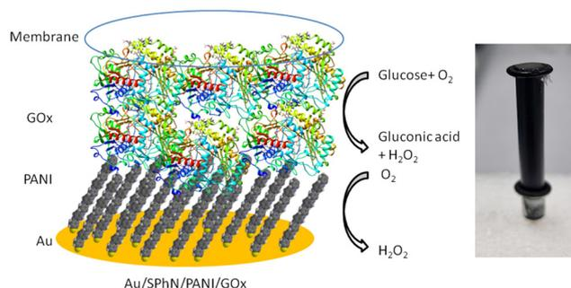
**Fig. 4** Schematic presentation and photography of the Au/SPhN/PANI/GOx bioelectrode with the reactions occurring in the corresponding layers.
