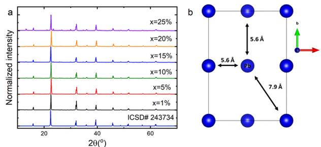
**Fig. 1** X-ray diffraction patterns of the CsPbCl<sub>3</sub>:x%Nd<sup>3+</sup> perovskite powders (a) and a simplified unit cell scheme of an undoped sample (b).
