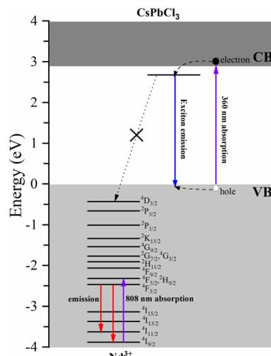
**Fig. 10** Electronic energy level scheme determined for the CsPbCl<sub>3</sub>:Nd<sup>3+</sup> perovskite powder.
