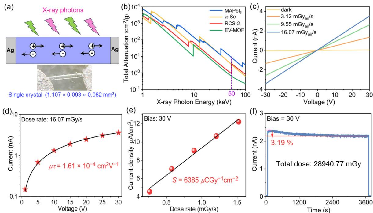
**Fig. 2** Single-crystal X-ray detection performance of RCS-2: (a) schematic illustration of the X-ray detector and actual electrode diagram. (b) Calculated mass attenuation coefficients. (c)  $I$ - $V$  curves under X-ray off and on with different exposed dose rates. (d) Voltage-dependent photocurrent curves fitted by the Hecht equation. (e) Photocurrent density versus dose rate measured at a bias voltage of 30 V. (f) Device stability in air under continuous X-ray irradiation.
