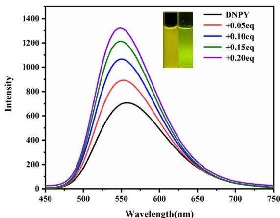
Fig. 1 Fluorescence emission spectra of DNPY with gradual addition of SBE- $\beta$ -CD in aqueous solution (inset: photographs of DNPY and DNPY-SBE- $\beta$ -CD). [DNPY] =  $1.0 \times 10^{-5}$  mol L $^{-1}$ .
