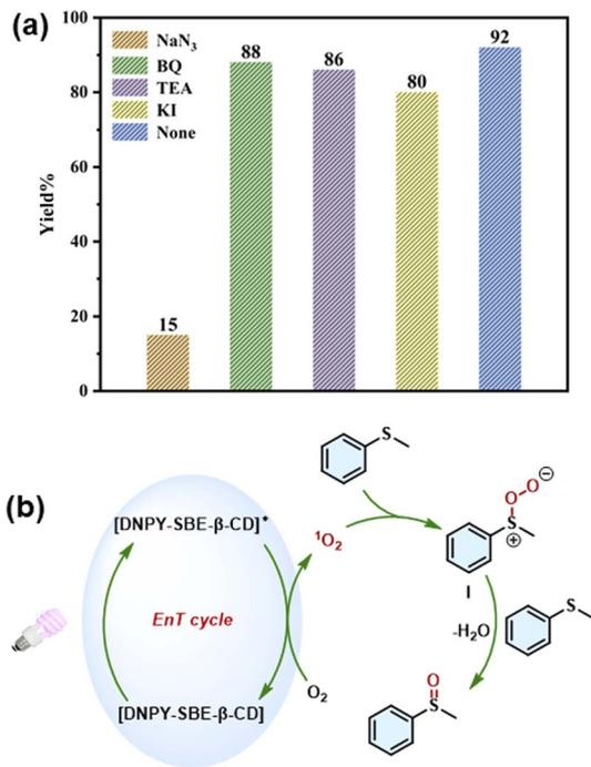
Fig. 3 (a) Control experiments for the thioanisole photooxidation reaction in the presence of different scavengers: NaN<sub>3</sub>, BQ, TEA, and KI. (b) The proposed mechanism for the photooxidation reaction of thioanisole.
