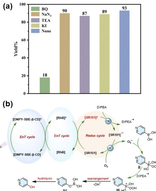
Fig. 6 (a) Control experiments for the oxidative hydroxylation of arylboronic acids in the presence of different scavengers:  $\text{NaN}_3$ , BQ, TEA, and KI. (b) The proposed mechanism for the oxidative hydroxylation of arylboronic acids.
