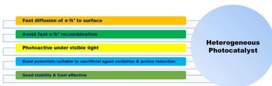
Fig. 4 Properties of heterogeneous photocatalysts.
