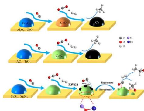
Fig. 7 Schematic of Co phase transformation during CO reduction and  $\text{CO}_2$  hydrogenation reaction on Na–Co catalysts supported on different supports. Reprinted with permission from ref. 71. Copyright 2020 Elsevier.
