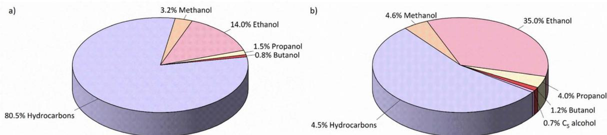
Fig. 4 Product distributions of CO<sub>2</sub> hydrogenation (a) 2% Na–Fe@C catalyst and (b) 2% Na–Fe@C/5% K–CuZnAl multifunctional catalyst (b). Reprinted with permission from ref. 25. Copyright 2021 American Chemical Society.
