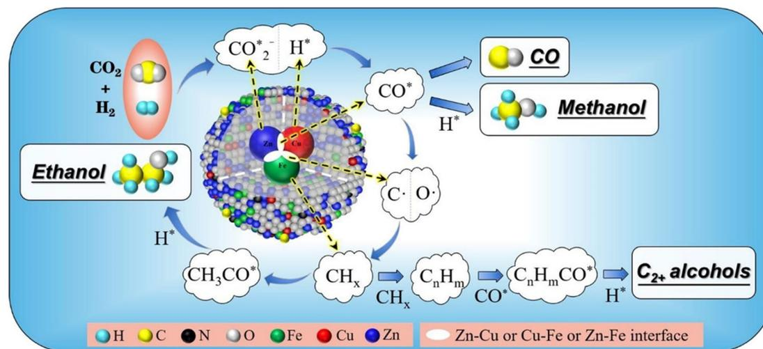
Fig. 8 The weak base of doped N promotes the generation of CO<sub>2</sub><sup>•-</sup> species through CO<sub>2</sub> activation, which is further regulated by the CuZnFe catalyst to form intermediates including CO\*, CH<sub>x</sub>, and HCOO\* species to form higher alcohols through CO\* insertion into C<sub>n</sub>H<sub>m</sub>. Reprinted with permission from ref. 16. Copyright 2022 Elsevier.
