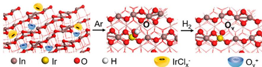
Fig. 3 Schematic illustration of synthesis procedure for Ir<sub>1</sub>-In<sub>2</sub>O<sub>3</sub> SAC. The diagram depicts the generation of O<sub>v</sub> by partially reducing In<sub>2</sub>O<sub>3</sub> under H<sub>2</sub> atmosphere prior to impregnating of the Ir. These O<sub>v</sub> then act as the anchoring site for single Ir atoms and promote the trapping of IrCl<sub>6</sub><sup>2-</sup>. Reprinted with permission from ref. 46. Copyright 2020 American Chemical Society.
