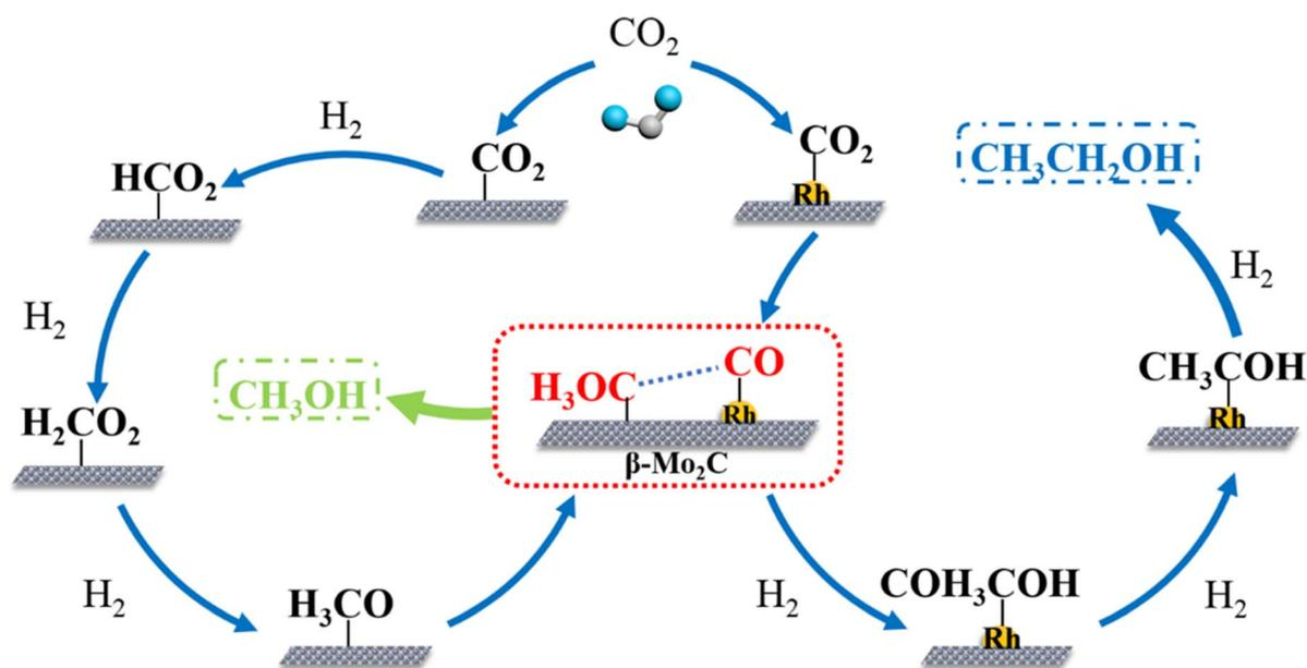
Fig. 12 Proposed reaction mechanism of  $\text{CO}_2$  hydrogenation to ethanol on the  $\beta\text{-Mo}_2\text{C}$  nanowires with a single Rh atom for promoting the C–C coupling mechanism and an introduction of an alkali metal K to regulate the balanced performance of the two active centers for improving the selectivity of ethanol. Reprinted with permission from ref. 53. Copyright 2022 Elsevier.
