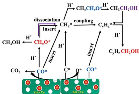
Fig. 11 Electronically modified Fermi level facilitates the formation of alkyl species to promote CO insertion with  $\text{CH}_x\text{-C}(\text{H}_x)\text{O}$  coupling for higher alcohols. Reprinted with permission from ref. 17. Copyright 2023 Elsevier.
