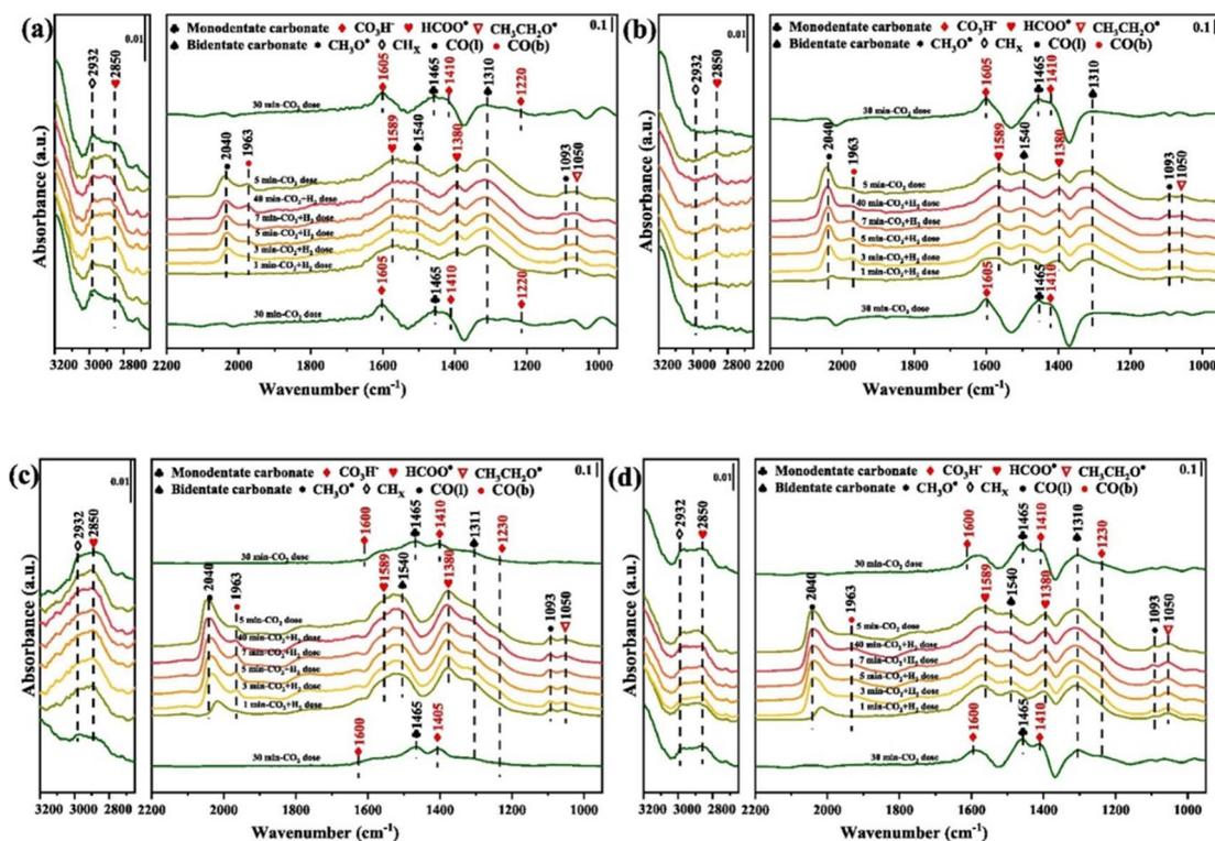
Fig. 6 *In situ* DRIFTS of various catalysts after switching the feed gas from CO<sub>2</sub> to CO<sub>2</sub> + H<sub>2</sub>, followed by returning to CO<sub>2</sub> at 250 °C and 0.1 MPa (a) 2Rh/CeO<sub>2</sub> (b) 2Rh0.5Fe/CeO<sub>2</sub> (c) 2Rh0.5Na/CeO<sub>2</sub> and (d) 2Rh0.5Fe0.5Na/CeO<sub>2</sub>. Reprinted with permission from ref. 51. Copyright 2024 Elsevier.
