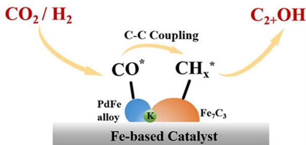
Fig. 9 Proposed reaction pathway that shows the non-dissociative activation of CO regulated by K and Pd to balance the dissociative activation of CO regulated by Fe<sub>2</sub>O<sub>3</sub> catalyst for promoting the C–C coupling mechanism. Reprinted with permission from ref. 26. Copyright 2024 American Chemical Society.
