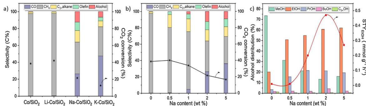
Fig. 5 Catalytic performance over Co/SiO<sub>2</sub> catalysts with different alkali metals and Na contents (a) CO<sub>2</sub> conversion and product selectivity with different alkali metals (b) CO<sub>2</sub> conversion and product selectivity Na contents (c) alcohol distribution and ethanol STY with different Na contents. Reprinted with permission from ref. 40. Copyright 2021 Elsevier.
