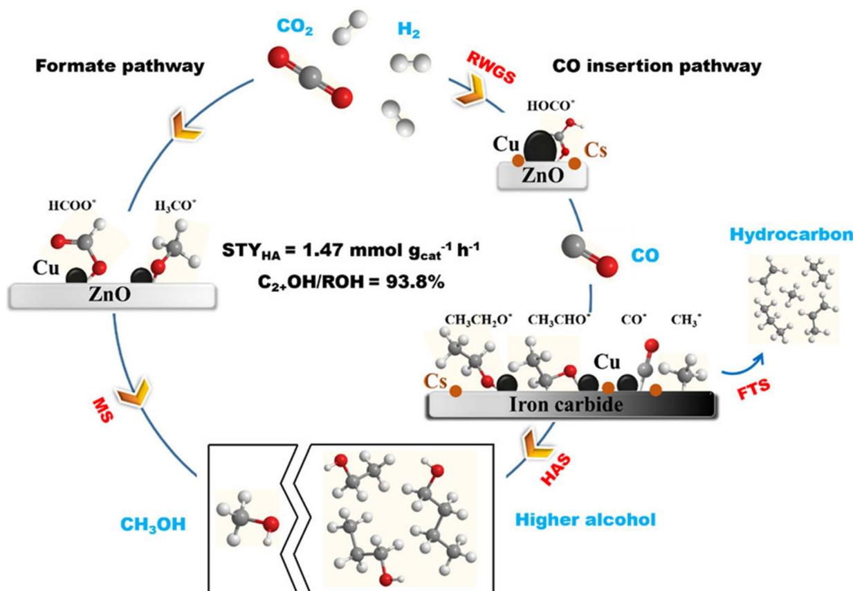
Fig. 10 Proposed reaction mechanism of CO<sub>2</sub> hydrogenation for higher alcohols through C(H)O\* insertion and CO insertion into hydrocarbons over Cs–CuFeZn catalysts. Reprinted with permission from ref. 37. Copyright 2020 American Chemical Society.
