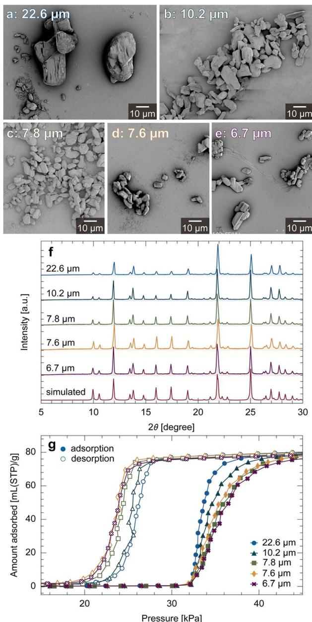
Fig. 2 (a)–(e) SEM images, (f) XRD patterns, and (g) CO<sub>2</sub> adsorption isotherms (273 K) of ELM-11 particles synthesized under various concentration conditions. The closed and open symbols in (g) represent adsorption and desorption branches, respectively.
