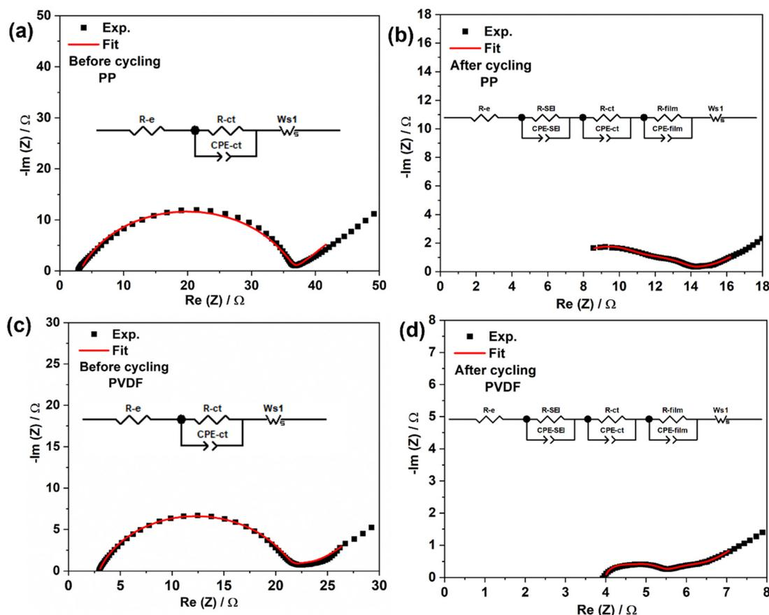
Fig. 5 Nyquist plots for LSB cells before and after cycling with (a), (b) PP and (c), (d) PVDF separators. The equivalent circuit parameters:  $R_e$  = electrolyte resistance,  $R_{ct}$  = charge-transfer resistance,  $R_{SEI}$  = resistance of solid electrolyte interphase,  $R_{film}$  related to  $Li_2S/Li_2S_2$  film, and  $Ws_1$ . CPE-ct, CPE-sd, CPE-SEI and CPE-film represent constant phase elements associated with  $R_{ct}$ ,  $R_{SEI}$  and  $R_{film}$  respectively.
