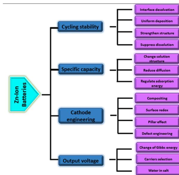
Fig. 10 Challenges in cathode materials for Zn-ion batteries.
